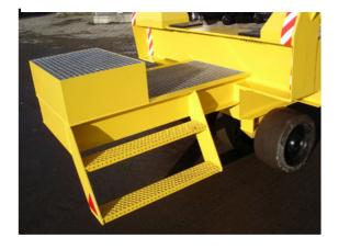
Steps and work platform in the back of trailer for cleaning and repair of the Spreader.
